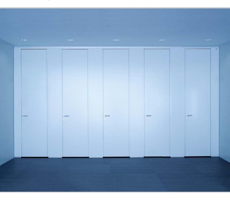
classiccell – privacy! The doors and pilasters are perfectly integrated into the washroom thanks to a shadow gap connection to the ceiling, walls and the floor. The wall connection is also available with u-profiles.
